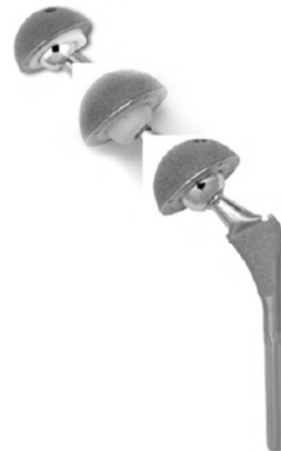
FIGURE II.5.6.10 Examples of the three types of bearing couples used in modern THA. From top to bottom: metal-on-polymer, ceramic-on-ceramic, and metal-on-metal (Linge™ line from Wright Medical Technology, Inc. Arlington, TN, USA).
